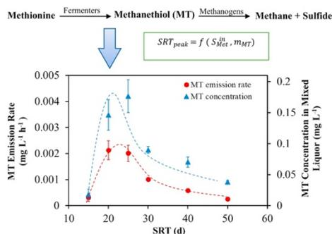
content in the feed sludge together with the large maintenance coefficient of MT fermenters are responsible for the peak MT emission emergence in the range of typical SRT used for anaerobic digestion. *Source: [Water Research, 138, 301-311](#)*
