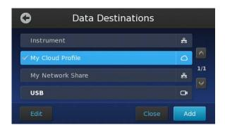
**Note:** Whichever destination you select, imaging data is also saved on the instrument, up to a limit of  $\sim$ 600 experiment files, after which the oldest files will be purged from memory and replaced with newer files.
