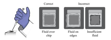
Note: A small amount of fluid running off the surface of the chip is acceptable.
