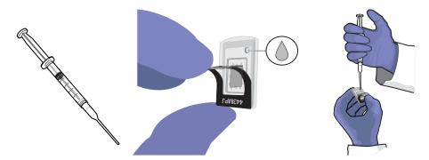
Figure 4 QuantStudio™ 3D Digital PCR Chip Lid v2
