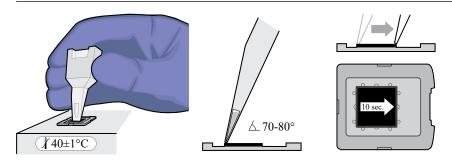
**d.** Confirm that the loading blade contains no residual fluid, indicating that the reaction has been completely loaded onto the chip.
