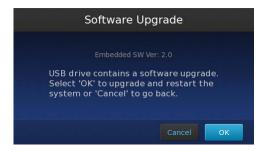
**IMPORTANT!** Do not remove the USB drive from the instrument until after the update is complete.
