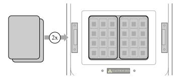
**IMPORTANT!** Make sure that each thermal pad is centered on the sample block and it completely covers the chips.
