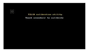
4. At the end of the calibration sequence, touch **OK** to save the new touchscreen calibration settings and restart the instrument.
