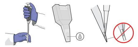
c. While holding the loading blade at a 70–80° angle relative to the heated block so that the port faces up, place the edge of the blade at the end of the chip. Adjust the angle of the blade until you visually confirm that it is wetting the chip. Then, in one smooth motion, slowly drag the blade across the chip while applying a slight downward pressure to dispense the reaction.
