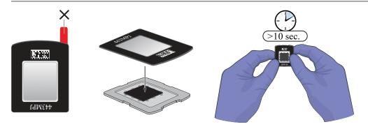
Proceed to filling the chip case with Immersion Fluid.
