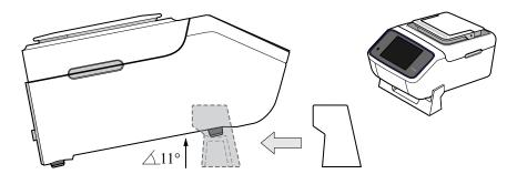
Open the heated cover and confirm that QuantStudio<sup>™</sup> 3D Digital PCR Chip Adapters are installed to both sample blocks.
