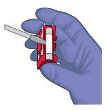
4. Replace each failed fuse with a 1.6A, Time-Lag T, 250VAC, 5 × 20-mm Fuse.
