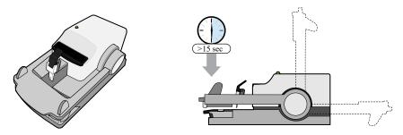
**IMPORTANT!** The loading arm requires >20 lbs of force to seal the lid. If you suspect that you are applying insufficient pressure, press down longer (>15 seconds).
