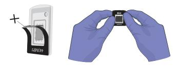
**IMPORTANT!** Press only on the label region of the chip lid. Pressure placed on the window of the chip lid can expel the PCR reactions out of the chip wells.
