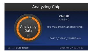
**Note:** If the run fails because the instrument is unable to read the chip, inspect the chip for problems and read the chip again. If the run fails repeatedly, discard the chip and prepare a replacement.
