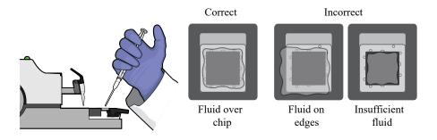
10. Rotate the loader arm so that the chip lid solidly contacts the chip. Firmly press down on the arm for 15 seconds to ensure a tight seal (you can count each flash of the status light, which flashes at 1-second intervals).
