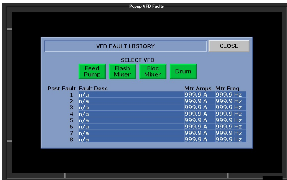
Figure 6.10 – VFD Fault Screen
