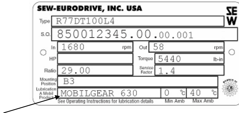
Figure 8.1 – ES35X Series Drum Drive Gear Motor Gear Box Name Plate
