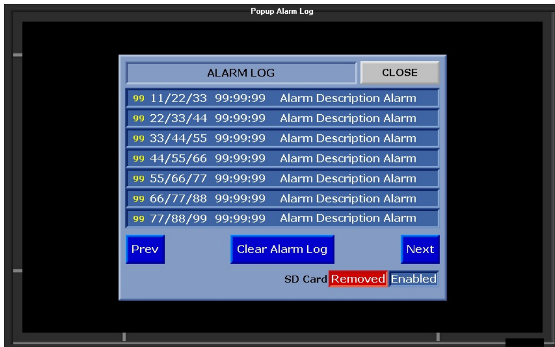
Figure 6.8 – Alarm History Screen
