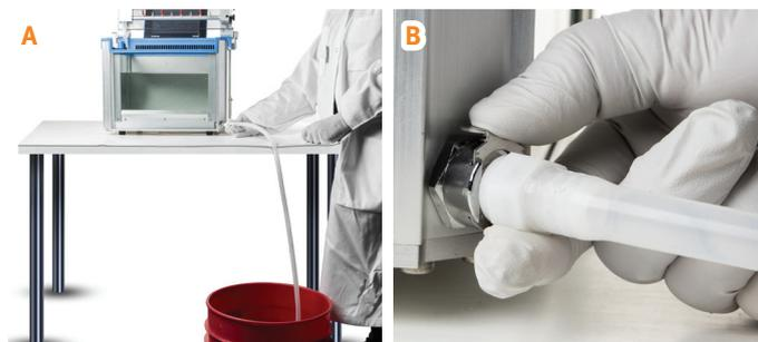
Figure 31. Connecting (A) and disconnecting (B) the drain tube.
