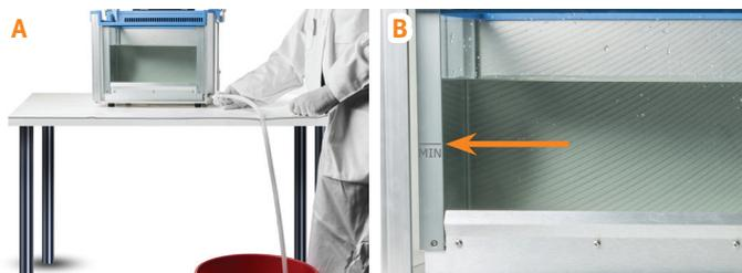
**Figure 17.** A: Insert the drain tube into a waste container before pushing in the drain tube connector into the DRAIN port. B: The minimum level on the water bath.
