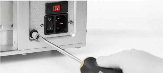
Figure 37. Removing the fuse holder.
