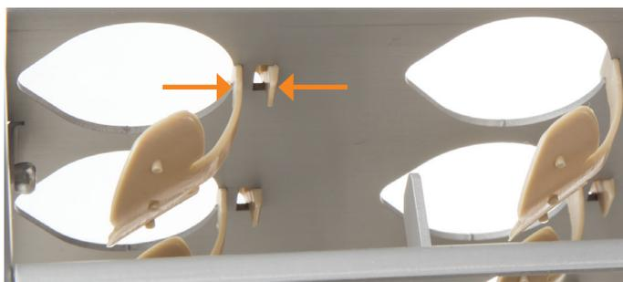
Figure 34. Releasing a vial spring.
