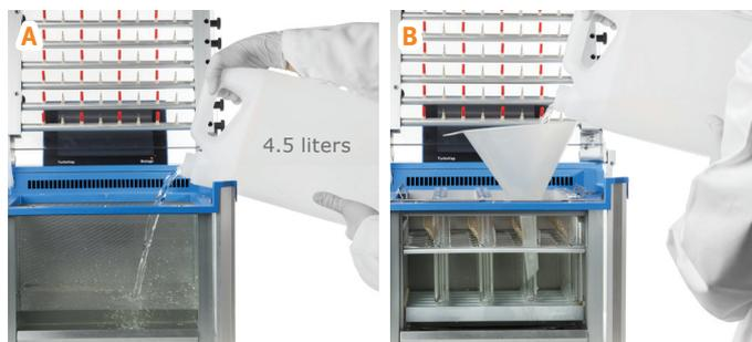
Figure 32. The water's surface must be above the minimum level marked on the water bath but not higher than just below the blue water bath top cover.
