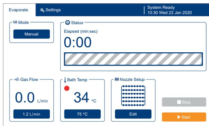
Figure 20. When the heater is on, a red, blinking dot is displayed in front of the current water bath temperature.
