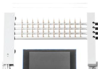
Figure 4. TurboVap P+ manifold with 48 nozzles.
