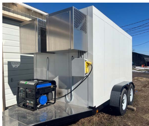
7'x12' refrigerated trailer (-18 °C ~ 10 °C)
