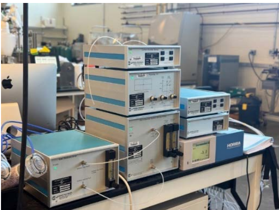
20-Channel Columbus Instruments Micro-Oxymax respirometer equipped with CO 2 , O 2 , CH 4 , and N 2 O sensors
